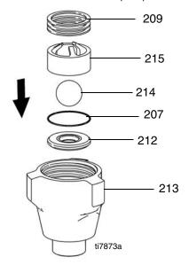
11. Place intake valve (213) assembly in vice. Install cylinder (205) assembly to intake valve. Torque to 350 ft-lb (475 N•m).
